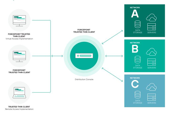
Security protections prevent data from being transferred between classification levels. The Distribution Console rejects all communications from unauthorized systems, reducing risk exposure to the enterprise.
