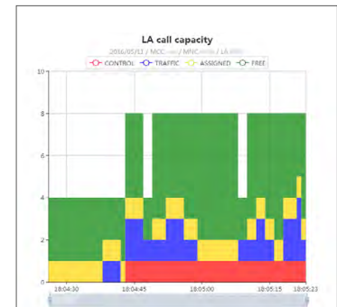
Call capacity (available and occupied slots) in a TETRA cell
